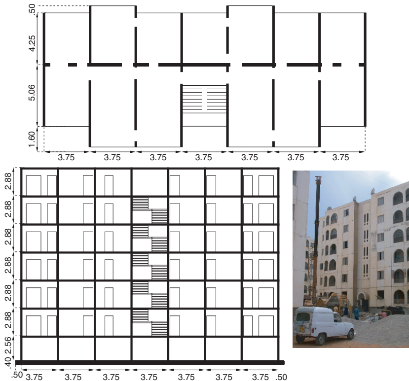
Fig. 3.4.2 Plan (upper), elevation (lower left) and view (lower right) of the studied COSIDER building. Values are given in meters
