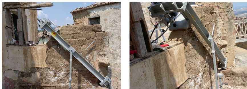
Fig. 4.5.7 Diagonal compression test
